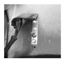
After the safety switch is mounted, connect to the Hood Safety Switch cable making sure that the connector is plugged in and <u>you hear 2 clicks</u>. If this isn't plugged in securely, it could come loose and could cause problems later. When finished, secure wiring to the truck frame.
